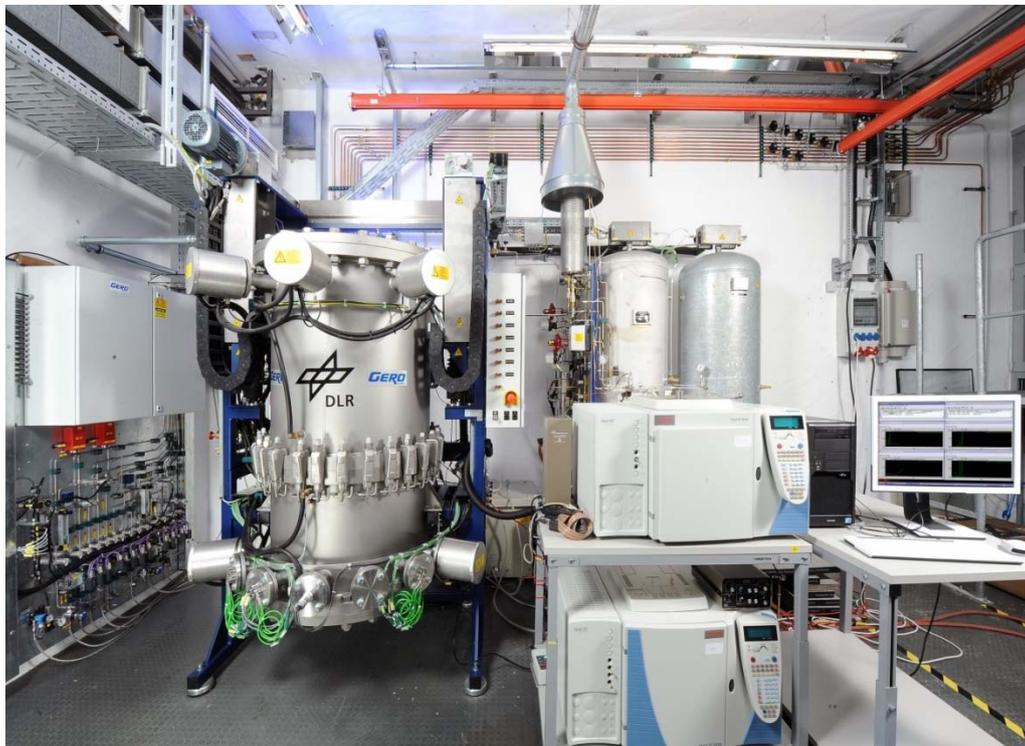
**Figure 1: Test rig for characterisation of 10 cell stack at elevated pressure.**
