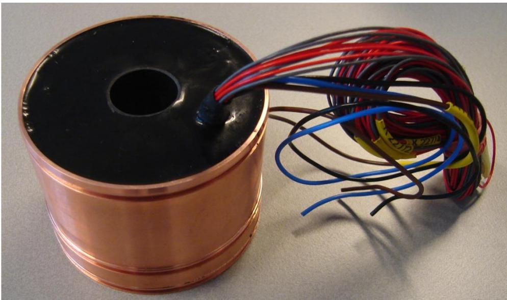
Figure 8: Manufactured stator with copper sleeve
