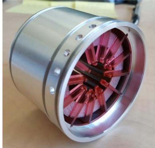
Figure 5: Assembled stator of the high-speed generator, with aluminium based cooling sleeve
