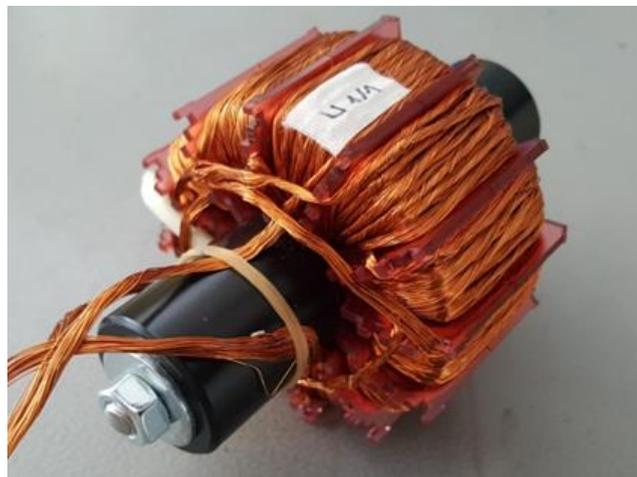
Figure 4: The stator of the high-speed generator during the manufacturing process
