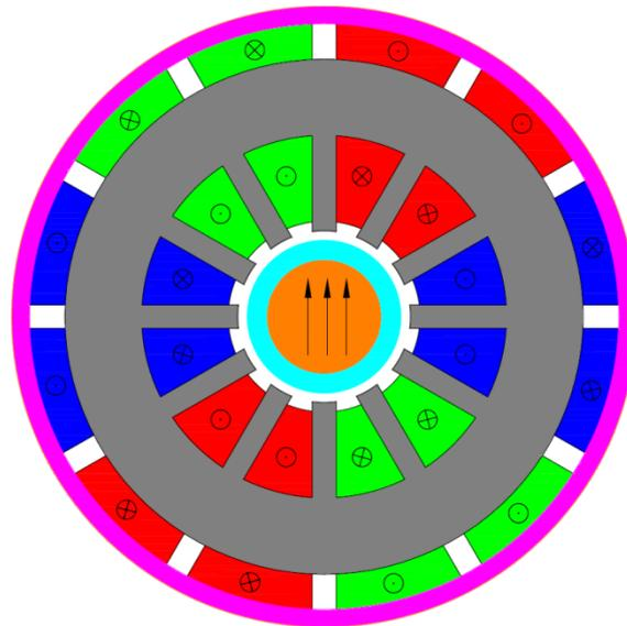
Figure 2: Adopted design of the high-speed generator
