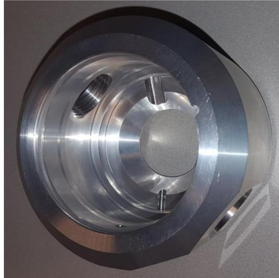
Figure 3: Housing for the new generator
