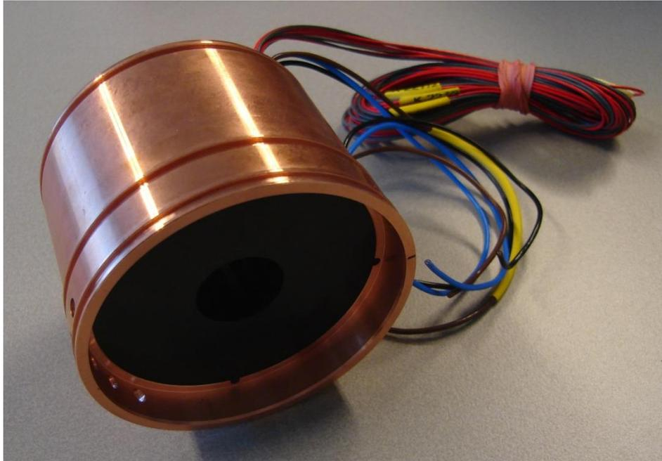
Figure 7: Manufactured stator with copper sleeve
