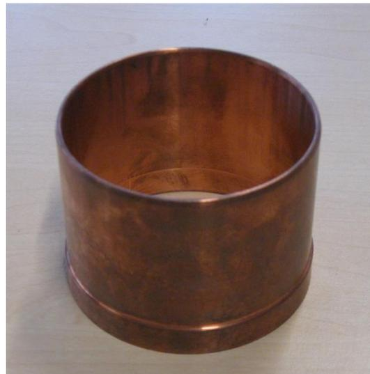
Figure 6: Copper sleeve of the high-speed generator, used in the final prototype
