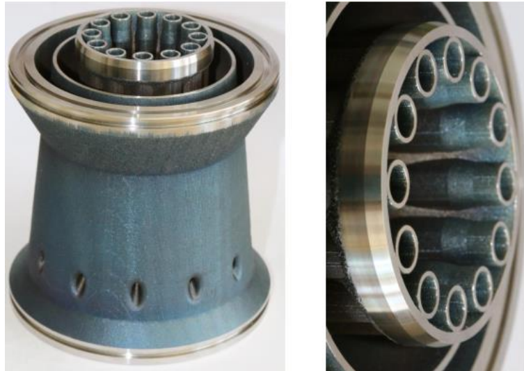
Figure 8: Combustor for integration into the test rig
