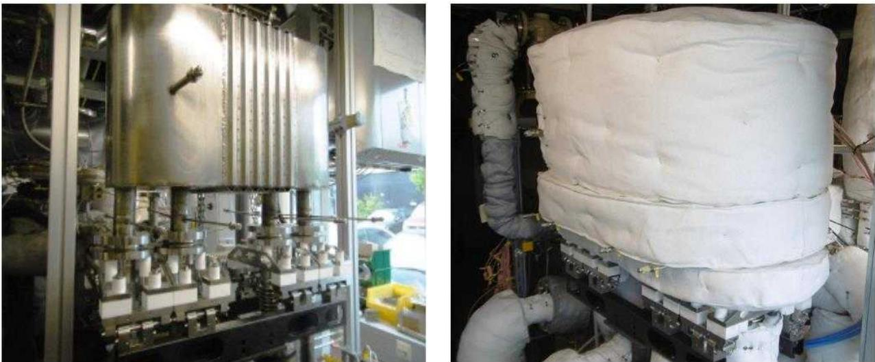
Figure 10: Optimized Recuperator from Hiflux integrated into MGT test rig: on the left without heat insulation on the right with heat insulation [15]
