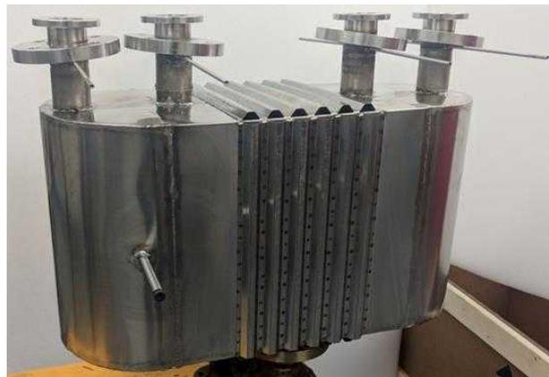
Figure 3: Recuperator for the top-performance layout
