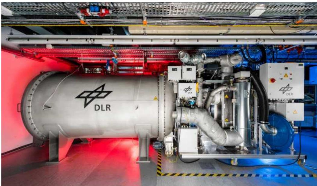
Figure 5: SOFC test rig of the top-performance layout
