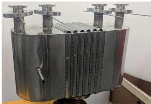
Figure 12: Newly manufactured recuperator [2]
